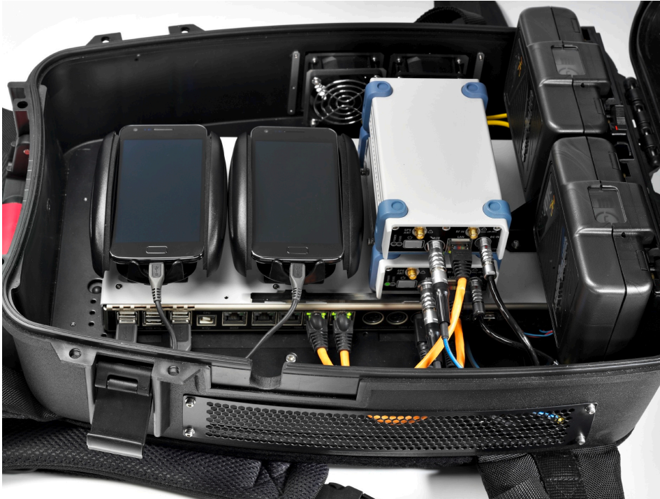
Fig. 3-1: R&S TSME-Z3: cable connections
